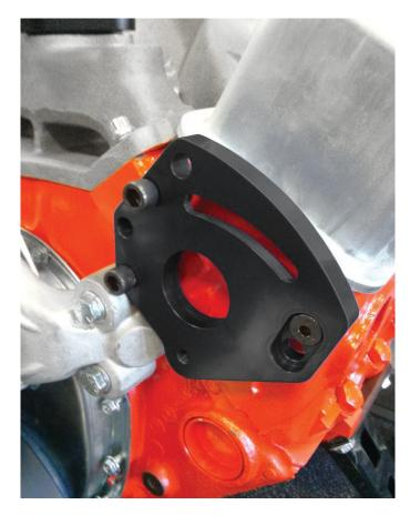
**8.** Rotate pump assembly until proper belt tension is reached and tighten the pump to bracket retainer bolts.
